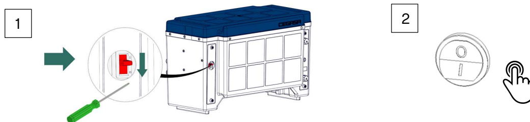
Figure 6-3. Disconnect the circuit breakers (CB) and leave the switch in the 'O' (OFF) position.
