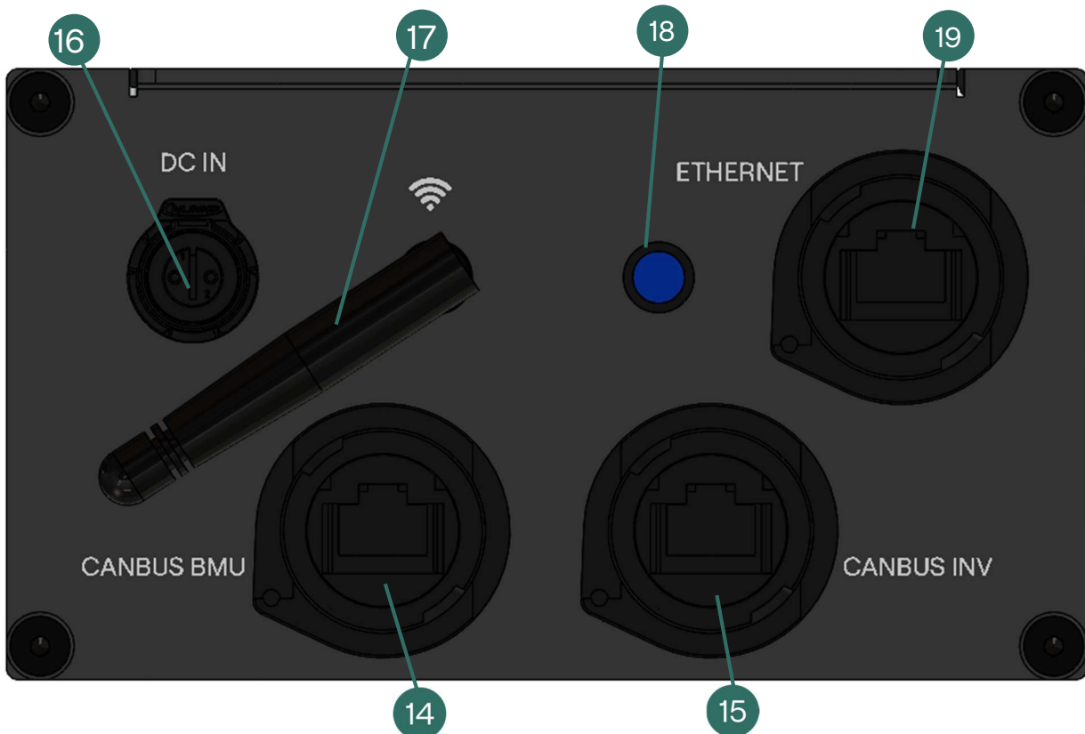
Figure 3-10. BMU rear with Master MCS.
