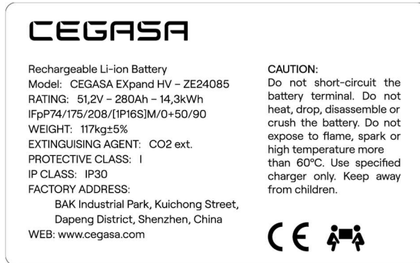
Figure 2-1. HV EXpand module - Rating plate 1.
